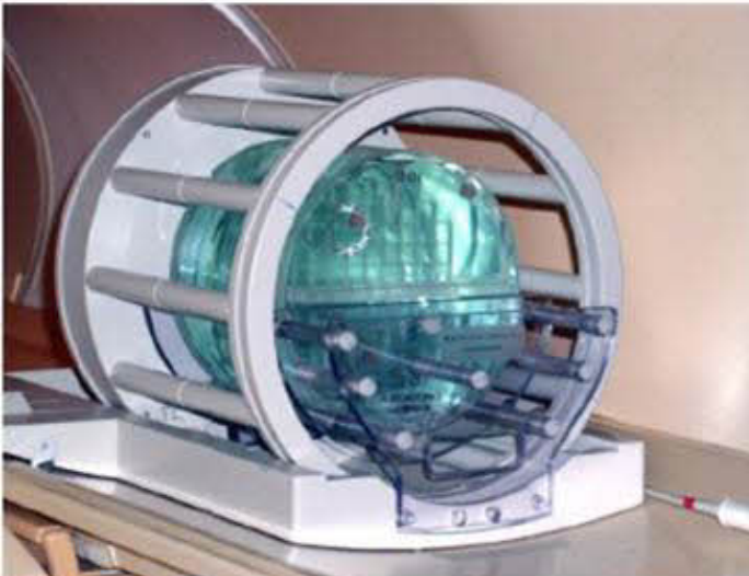
Fig. 2: This is the multimodality phantom that it is used for the measurements in the MRI course.
