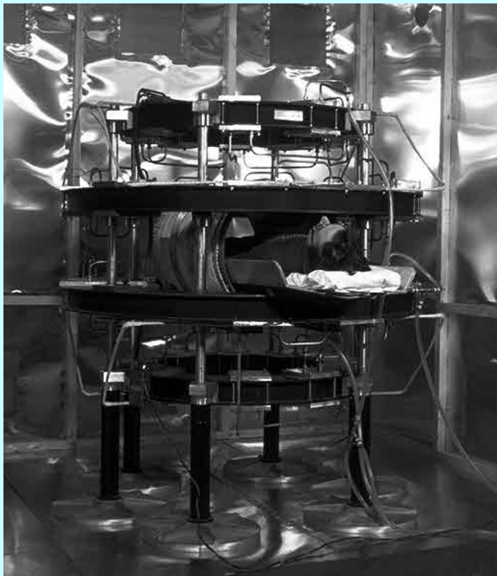
Fig. 1: Photo of the first MR Imager capable of producing clinical whole body Images at Aberdeen..
