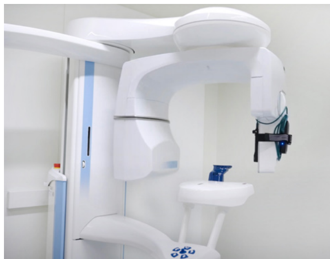
Figure 2. Recommended mounting of Mako for CBCT and panoramic systems
