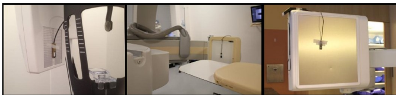
Figure 5.2. Position of a flat solid-state probe to measure the K_{a,i} (FDD) in a dental CBCT (left), a C-arm for angiography CBCT (right) and a CBCT in radiotherapy. Used with permission from F. Schöfer, B. Renger and K. Mair, respectively.
