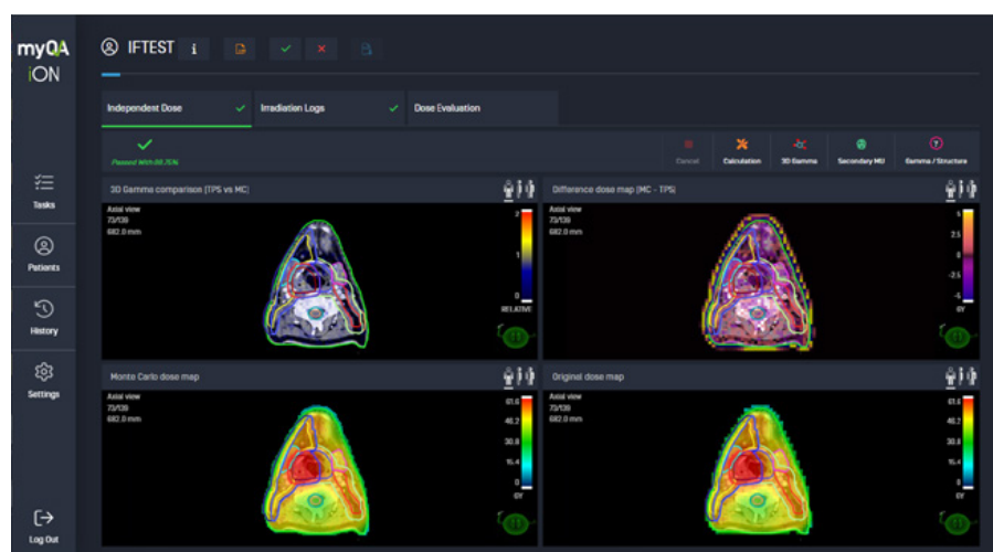
Figure 1. Independent dose evaluation: Monte Carlo calculation compared to TPS calculation with 3D gamma analysis on patient CT.
