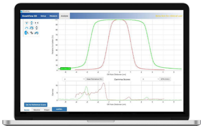
Figure 2: DoseView Software displays scan comparisons with visual overlays and gamma comparisons against the selected reference scans.
