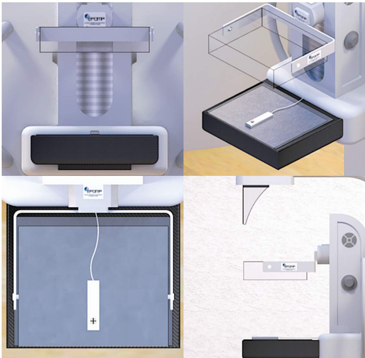
Figure 30 Schematic showing the setup for the measurement of K_m .
