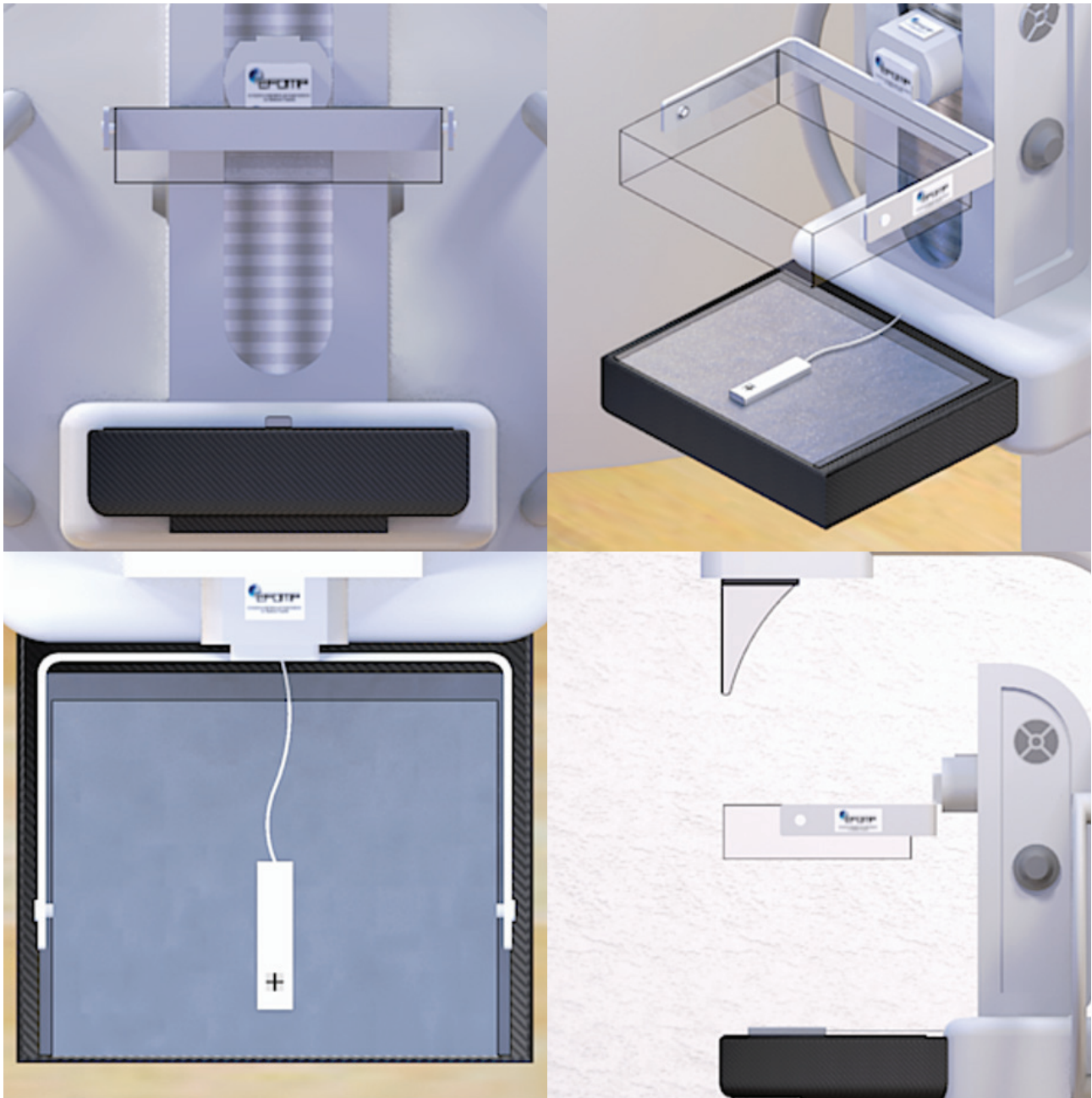
Figure 4 Setup for the tube output test
